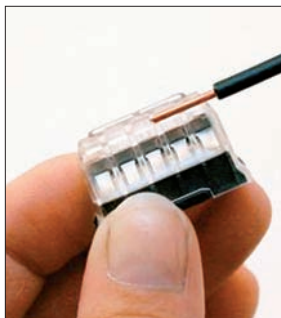
Insulation removal 8 - 9 mm
