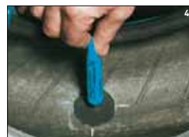
Spread the solution over the buffed area. Leave 5 mins to dry. Put a drop of solution in the hole's channel.
