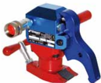
Delivered with removable magnetic base to increase stroke by 20 mm
