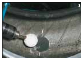
Lightly buff, until curing-bladder pattern disappears and remove dust. [Tool turns between 1500 and 5000 rev/ min max].
