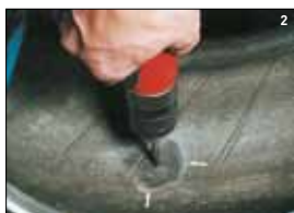
Measure the injury to choose the correct PRP. Drill out the puncture to size from the inside, at the correct angle. [Tool turns at between 1500 and 5000 revs/ min max].
