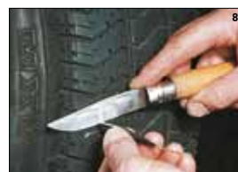
After remounting and inflating, cut (without pulling). [On the sidewall, leave 1 or 2 mm for rivet consolidation effect].
